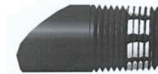
APPLY A MODERATE AMOUNT OF PIPE COMPOUND TO PIPE ONLY (LEAVE TWO END THREADS BARE),
